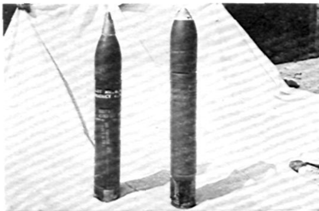
M-16 spin-stabilized rocket on left and the M-8 fin-stabilized rocket on the right.
