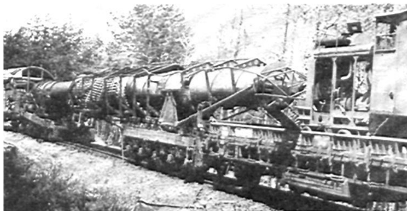
Tube No. 1 as viewed from gondola carrying cradle. Note burned-out framework of gondola that carried accessories.
